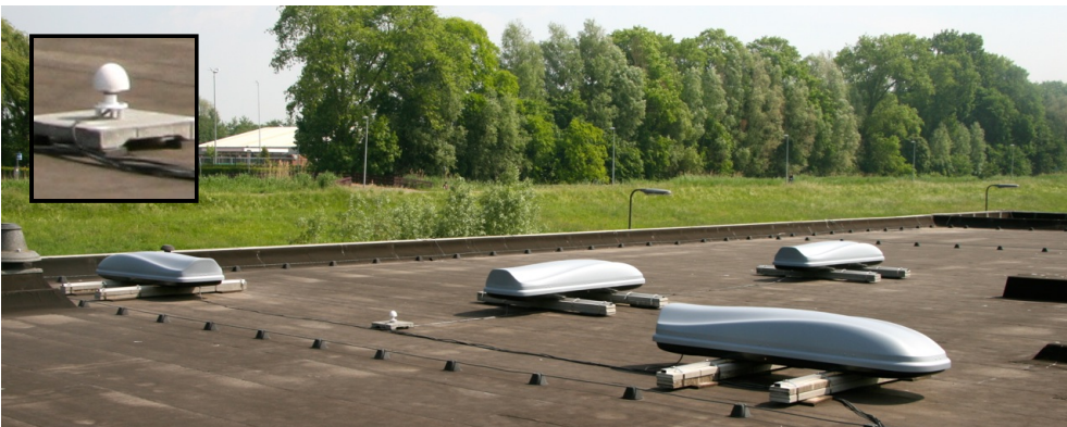
Figure 2.12 – The four-detector HiSPARC station (Figure 2.11) at TeleCity, Amsterdam Science Park. Each detector is placed in a roof box for protection against the elements. The inset shows a close-up of the GPS antenna.
