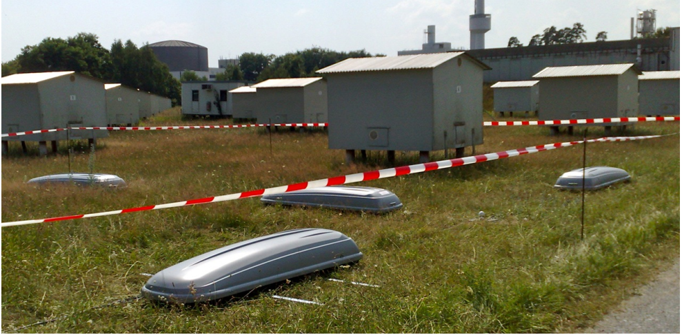
Figure 5.2 – HiSPARC station at the KASCADE experiment. The roof boxes contain the HiSPARC detectors. Several KASCADE detector huts are visible in the background. The large building in the background on the right is the central calorimeter and electronics building.
